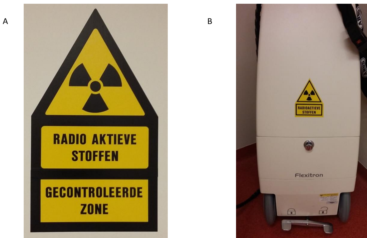
Figure 4.1 A: the warning sign for ionizing radiation and underneath the rectangular signs, with black edge, with the text 'RADIOACTIEVE STOFFEN' and 'GECONTROLEERDE ZONE'
