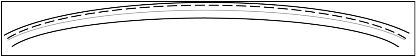
Figure 2.1: Path deviation in transfer tube: the actual source path (---) deviates from the ideal source path (—).
