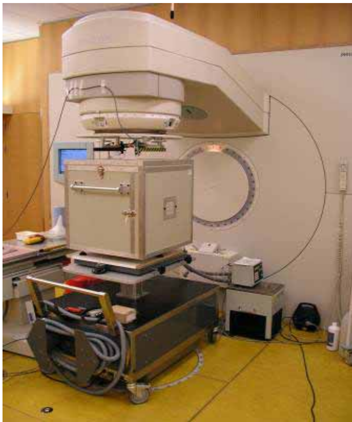
Figure 1: Setup of the portable NMI water calorimeter in a clinical photon beam
