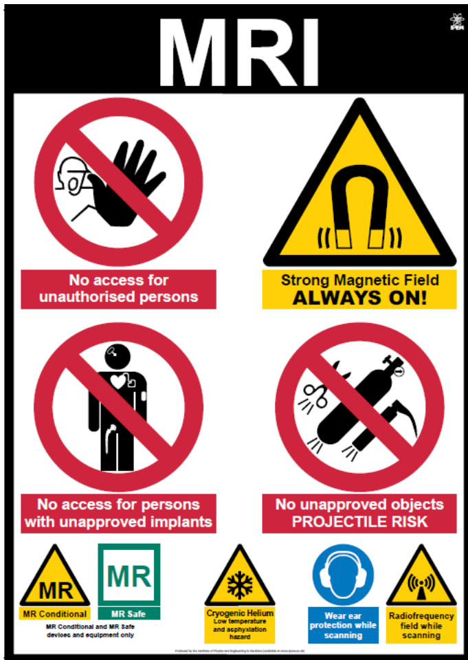
Figure 4: Example signs for an MRI scanner room, indicating the various hazards. The IPEM offers free downloads of MRI safety notices [63].
