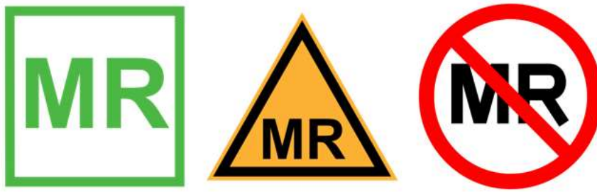
Figure 5: U.S. FDA labelling criteria (developed by ASTM and included in IEC-62570) for devices taken into the scanner room [60]. These figures are redrawings from Wikimedia Commons [64]. Green square: MR Safe; yellow triangle: MR Conditional; red circle: MR Unsafe.
