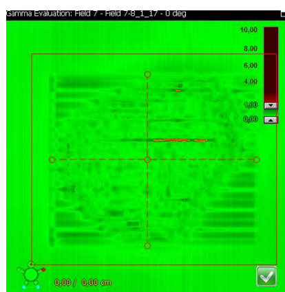
Figure 3.4 b Example of a field with a tongue and groove effect dose discrepancy.
