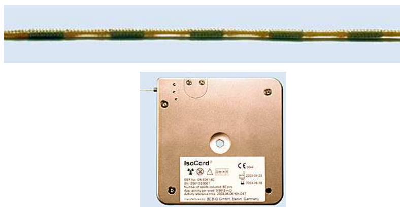
Figure 4: Close-up of IsoCord strand (top) and the cartridge (bottom).
