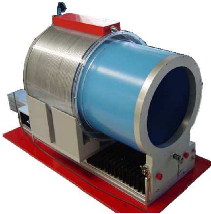
Figure 12: The GROVEX extrapolation chamber maintained at PTB
